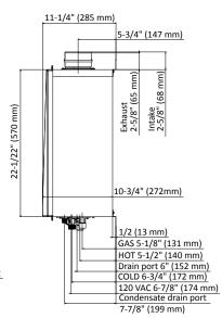
Thicker heat exchanger drum and utilizes commercial-grade copper for the heat exchanger tubing. Provides a variety of installation options: outdoor, and direct vent. Complies with SCAQMD Rule 1146.2 and other air quality management districts with similar NOx Emission requirements of 14 ng/J or 20 PPM. Easy-Link System capable up to 4 units. Multi-Link System capable up to 20 units.
